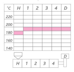
HF123 should be processed on equipment designed or retrofitted for LLDPE, i.e.
