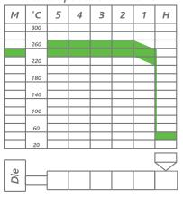
Cooling water (chill roll): 15-30°C Cooling water (water bath): 15-40°C Cooling water (monofilaments): 60°C
